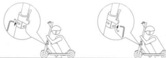
If your standpipe in the electric scooter is shaking, please use the M5 hex wrench to lock the two screws at the folding mechanism.
