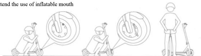
If your electric scooter front and rear tires are deficiency, please use the extended inflatable mouth to connect the car body tires to cheer. First remove the front and rear tire inflatable mouth cap, and then tighten the extension of the inflatable mouth and tire inflatable mouth, and connect the pump to inflate after they are to be tightened.
