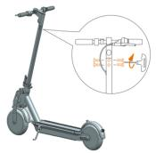
2. Firmly connect the wires inside the handle and the stem. Slide the handle onto the stem. Be aware of the correct orientation.
