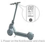
. Power on the KickScooter and check the power level indicator. Charge the KickScooter if the battery level is low.
