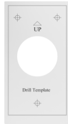
Drill Template for Intercom Panel (x1)
