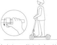
3 After electric scooter slide, the other foot pedal, when feet remain stable, tap the port finger (to be 5km / h above the speed will start the throttle)
