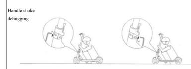
If your standpipe in the electric scooter is shaking, please use the M5 hex wrench to lock the two screws at the folding mechanism.
