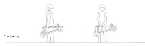
After folding, hold the standpipe with one hand or both hands to transport.
