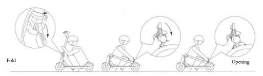
Make sure that the electric scooter is turned off, standpipe will dip through folding, open the folding wrench, and aim a the bell position and hook the bell with the rear mudguard. When opening you need to press the bell hook at the hook until the bell hook is out of the stall after the hook, the vertical straight standpipe and lock folding plate back to fold.
